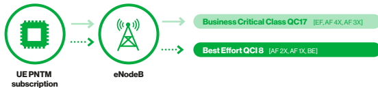
Figure 4. TOS/DSCP—aware bearing binding
