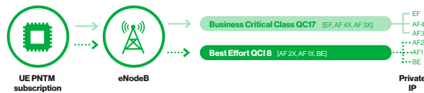
Figure 5. Private Network Traffic Management and Private IP classes mapping
