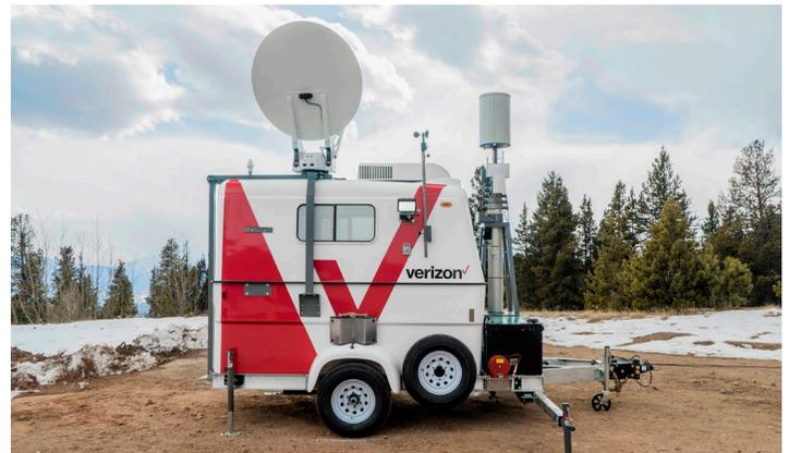
A Mobile Connectivity Trailer enables rapid creation of a cellular coverage area.
